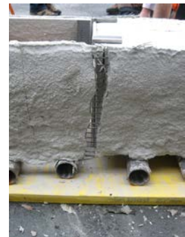
Figure 5: Test Specimen after pull-out test
