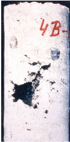
Figure 13: Spray voids behind steel reinforcing
