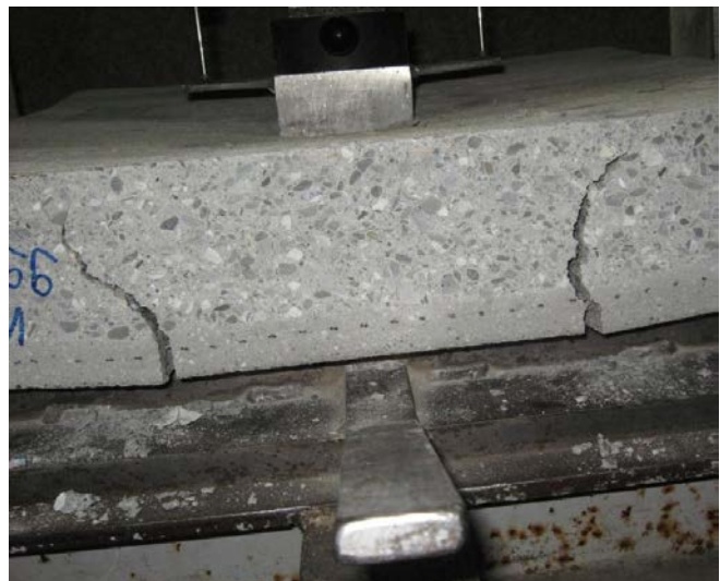
Figure 8: VSH test specimen at failure
