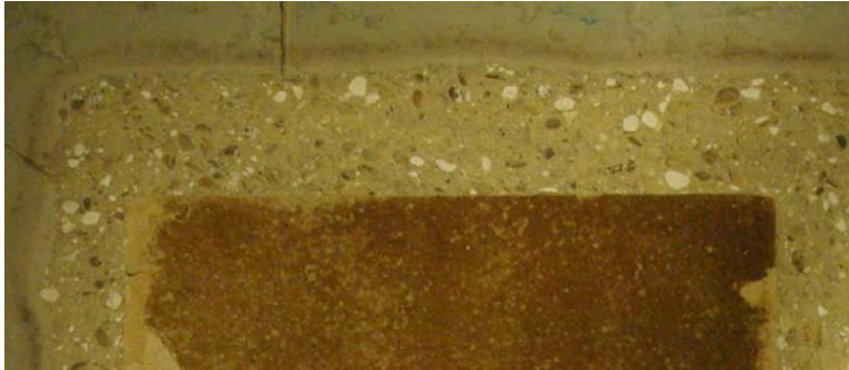
Figure 33: No spalling of the structural surface occurred as the concrete was laced with PP fibers
